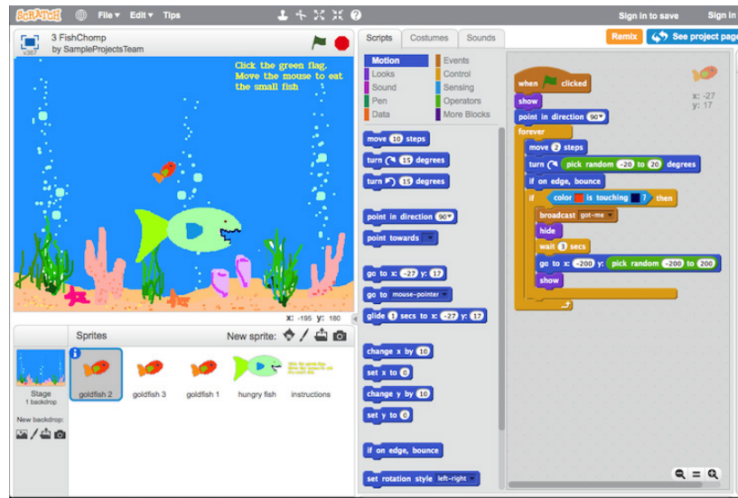
fig 8. The Scratch programming environment uses colored blocks that the user can drag-and-drop to write code. (image source: lk.media.mit.edu )
